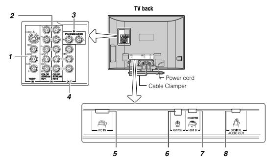
VIDEO-1 IN — Standard (composite) video and standard audio inputs plus optional S-video inputs for connecting devices with composite video or S-video output.
